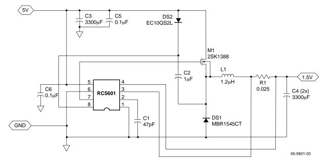
Figure 1. RC5601 Standard Test or Application Schematic for 5.5A, 1.5V Load
